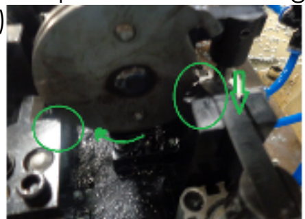
Modified Fixture (Assembly & machining reference same, & avoid wrong loading )
